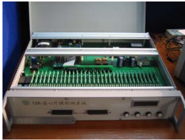
Figure 2. A photograph showing the amplifier (lower) and A/D converter (top middle). This side contained 64 isolated amplifier channels and another 64 channels were on the posterior side of PCB.
